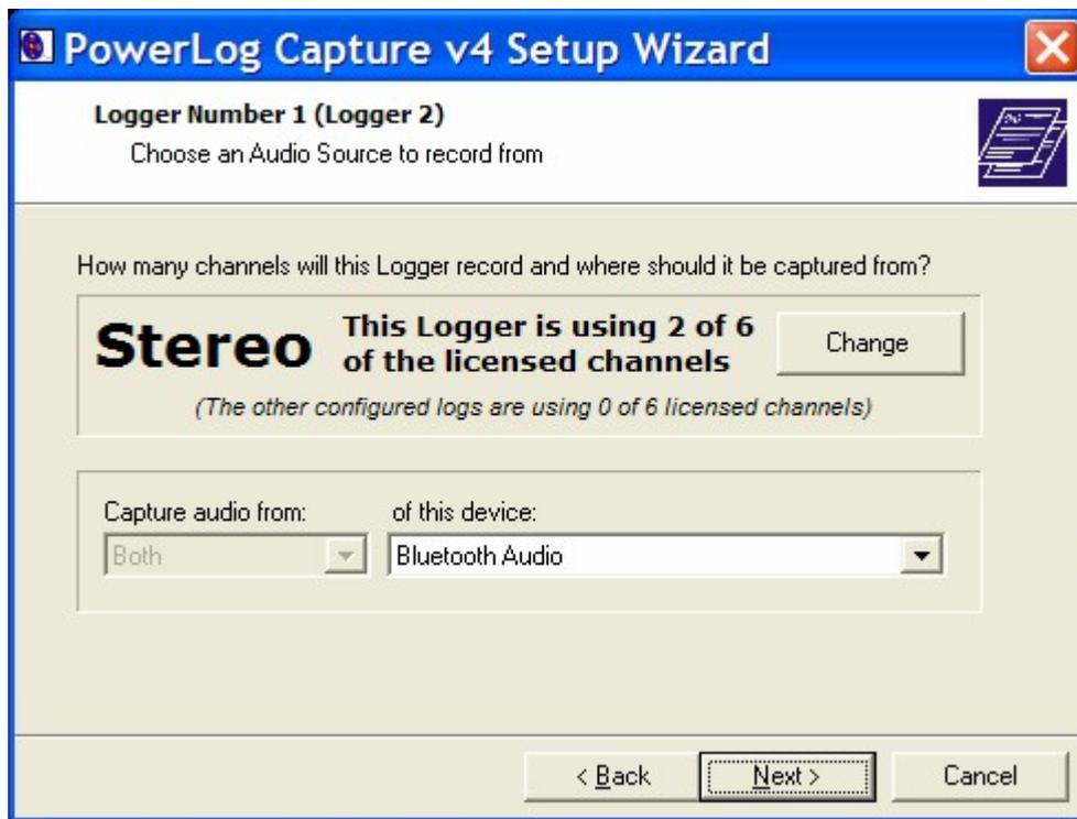
To change this log from a mono to a stereo or vice versa, click change, as indicated on the arrow diagram below.
