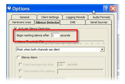
You can also change the volume threshold; this is at what volume your audio can drop below (in percentage terms) before PowerLog classes it as silence. To change it, move the Volume Threshold bar across or left or right.
