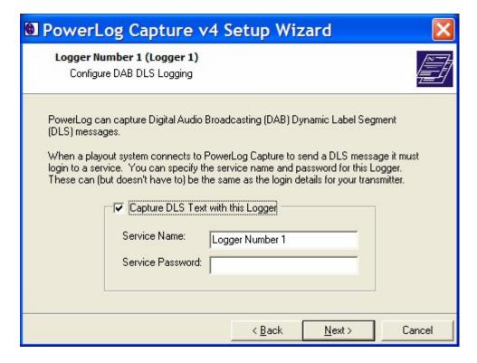
In order for PowerLog Capture to be able to receive DLS text it needs to be connected to your Playout system or an external source.
