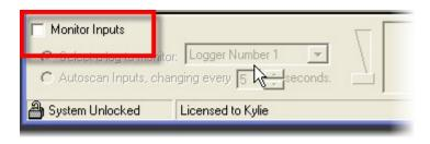
If the Monitor Inputs section is ticked you can listen to one of your logs as it is being recorded. This is especially useful to make sure that the audio coming into your PowerLog Capture machine is ok.
