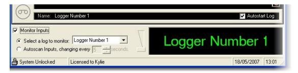
The default setting is set to only allow you to click on monitor inputs when your PowerLog Capture machine is unlocked. This can be changed by clicking on Settings > General > System Lock.
